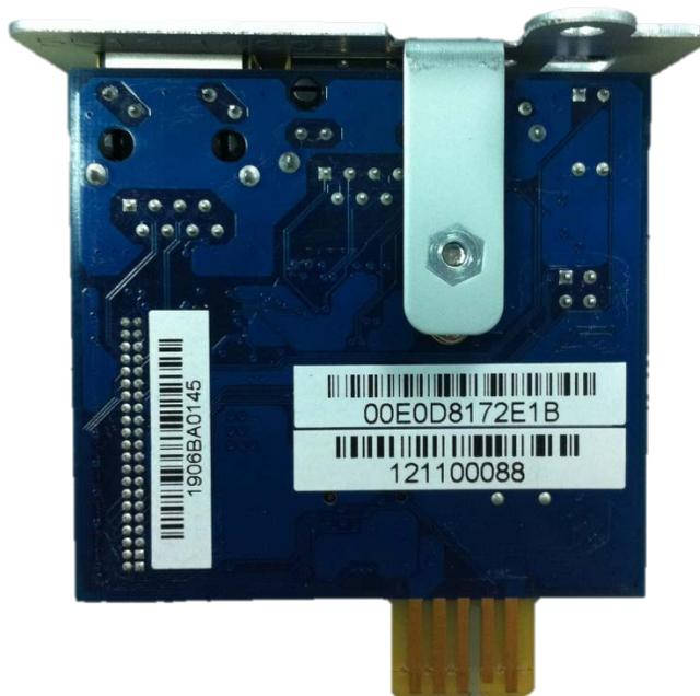
**Figure 14: RemotEye III MAC Address Label**
