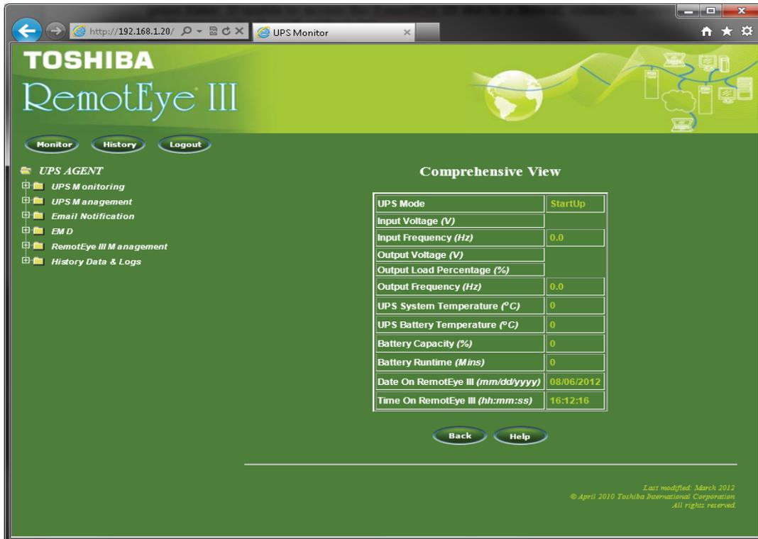
Figure 29: RemotEye III with Internet Explorer Example
